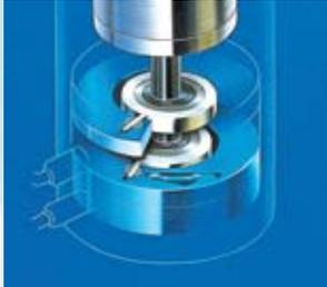
The design of the swing compressor reduces friction during operation for smoother and quieter rotation with less vibration resulting in a more durable compressor. It also minimizes the leakage of refrigerant gas during compression. The result is a system that operates quietly and efficiently.
